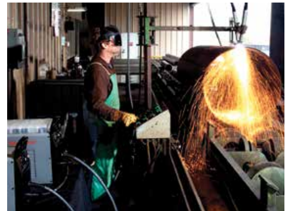
Pipe cutting and beveling
